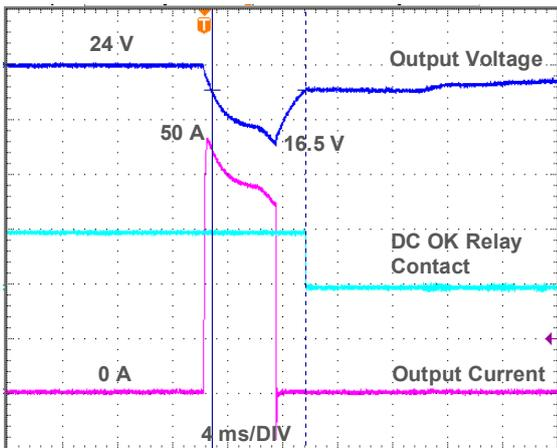
Fig. 8.3 APB 500% of nominal output current for 5 ms
