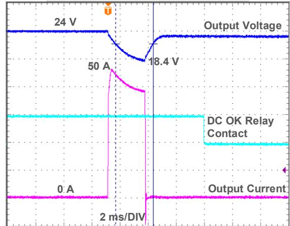
Fig. 8.2 APB 500% of nominal output current for 2 ms
