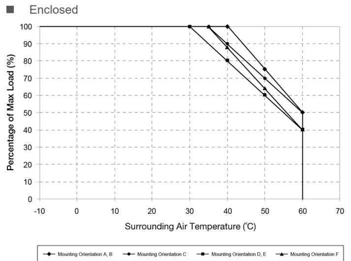
Fig.1.2 De-rating for Mounting Orientation A, B
