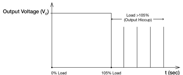
Additionally, if the  $I_o$  is  $< 105\%$  but  $> 100\%$  for a prolonged period of time (depending on the load), the Over Temperature Protection (OTP) will be activated due to high temperature on critical components. The power supply will then go into latch mode until the fault is removed and the mains is reapplied.
