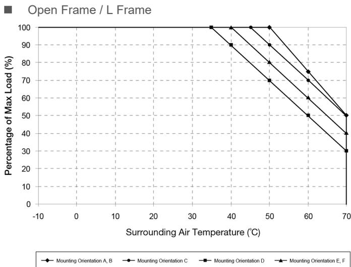
Fig.1.1 De-rating for Mounting Orientation A, B
