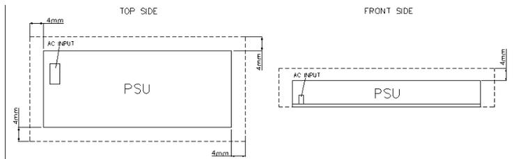
For safety reasons, please ensure the mounted device is kept safety distance as below at all sides from other components and equipments.
