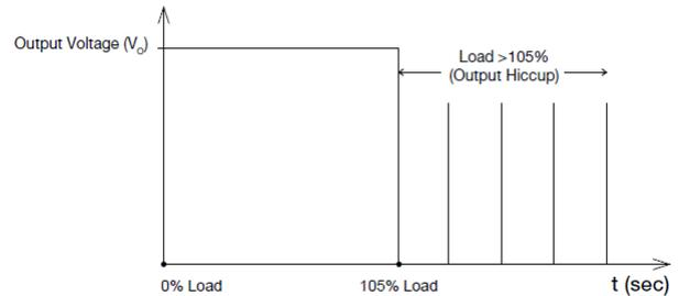
Additionally, if the  $I_o$  is  $<105\%$  but  $>100\%$  for a prolonged period of time (depending on the load), the Over Temperature Protection (OTP) will be activated due to high temperature on critical components. The power supply will then go into latch mode until the fault is removed and the mains is reapplied.
