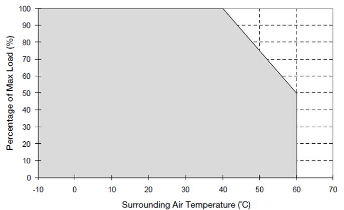
Fig.1.2 De-rating for Mounting Orientation A to F
