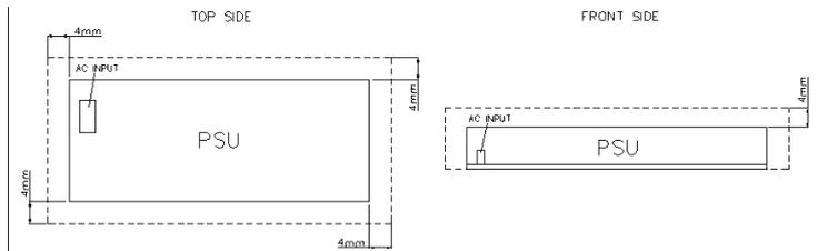
For safety reasons, please ensure the mounted device is kept safety distance as below at all sides from other components and equipments.
