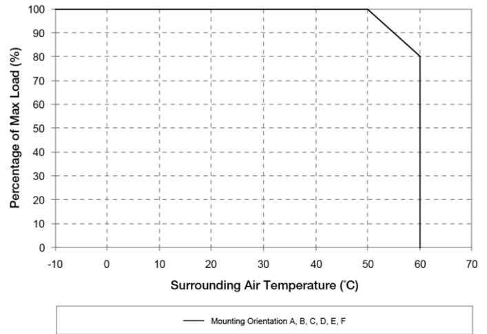
Fig.1.3 De-rating for Mounting Orientation A to F
