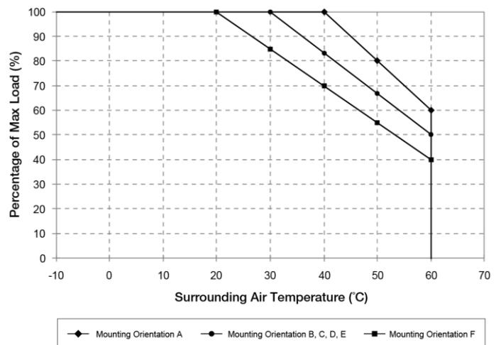
Fig.1.2 De-rating for Mounting Orientation A
