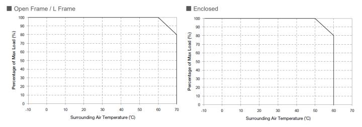
Fig.1.3 De-rating for Mounting Orientation A to F > 60°C de-rate power by 2% / °C
