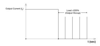
It is not recommended to prolong the duration of  $I_0$  when it is <220% but >100%, since it may cause damage to the PSU.
